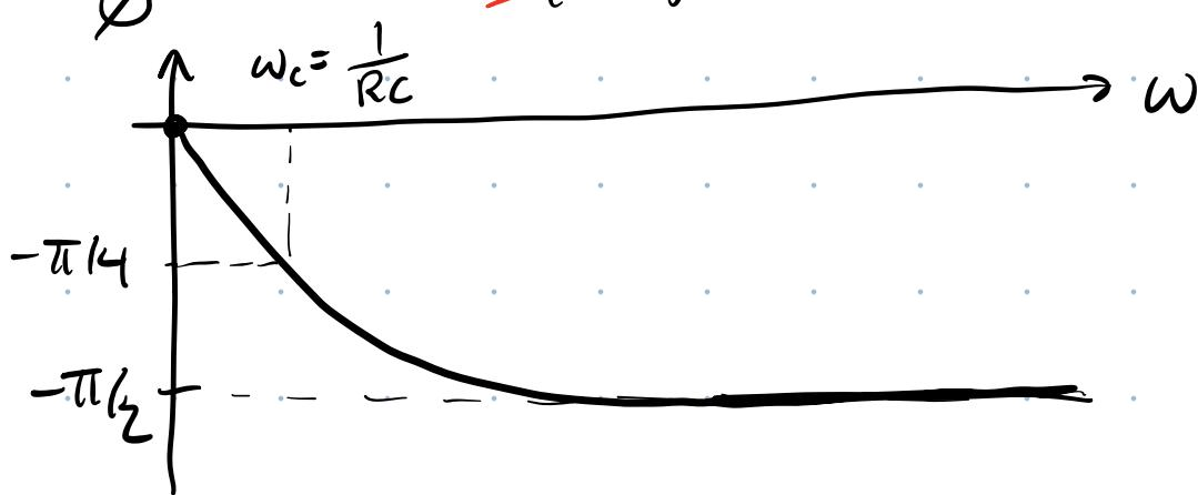
∴ Not only does this RC circuit attenuate signals at high frequencies, it also introduces a phase shift that approaches  $-\pi$  as frequency increases.
