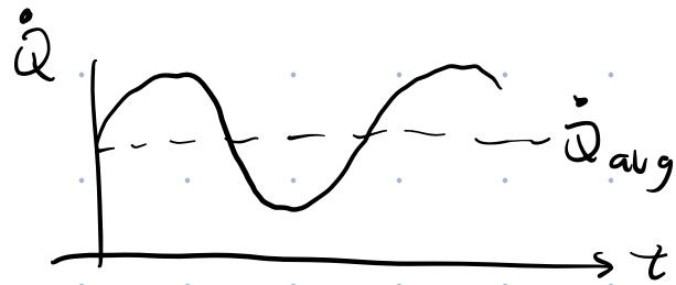
In such a scenario, there would be a temp. osc. on top of some avg. temp. gradient along the length of the copper rod.
