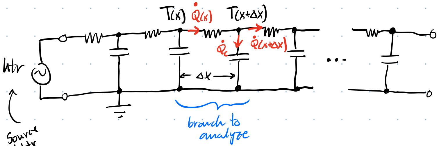
Distributed circuit model of Cu rod.
