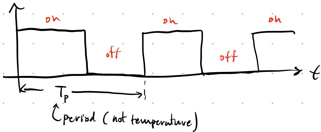
We know that square waves are made up of a sum of sine waves at frequencies of  $\frac{1}{T}, \frac{3}{T}, \frac{5}{T}, \dots, \frac{n}{T}$  (all the odd harmonics).
